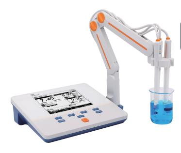
BEP - M300F: pH Electrode, Conductivity Cell (K=1), DO Probe, ATC Probe, Electrode Holder, pH Buffer Powders (4.01, 7.00, 10.01).
